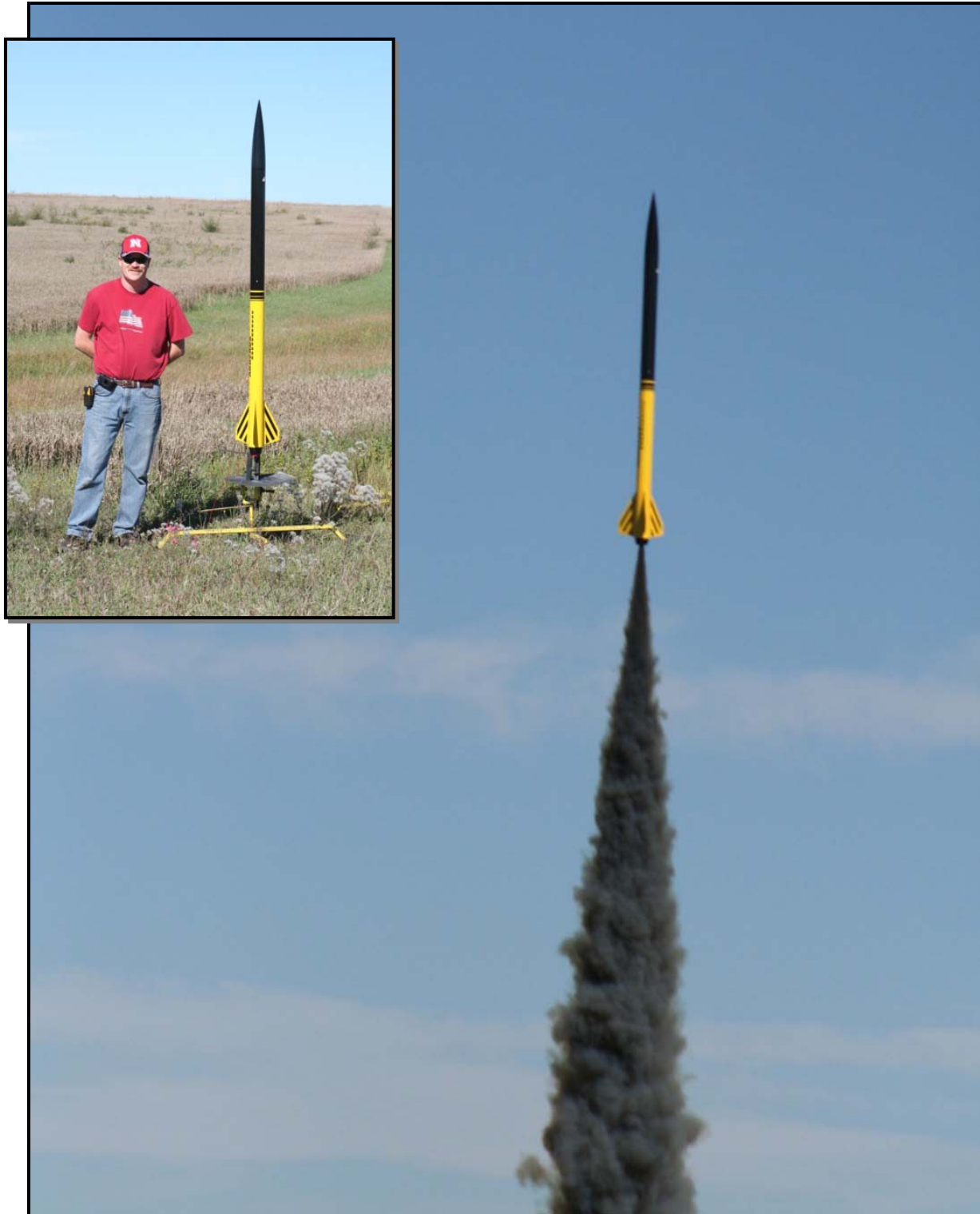
Joe Michel's upscale of the AeroTech Arreaux heads up to an altitude of 8,200' on a Pro54 K530.
