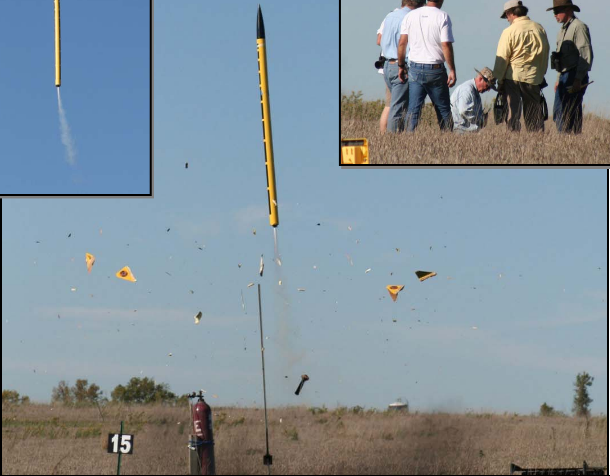
Denis Gilbert's Super Bee was severely damaged as a result of its HyperTek K240 catoing.
