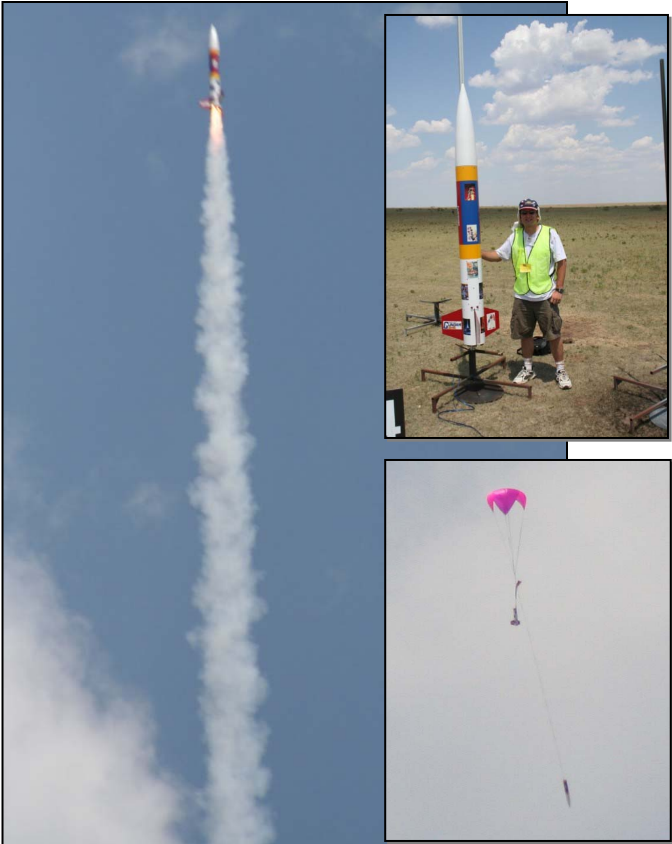
Richard Burney (the author) flew his rebuilt Mobile Rocket Gundam with a Pro54 L730 and three Pro38 I285's which started in midair. It reached an altitude of 6,461 feet. My greatest rocket achievement!
