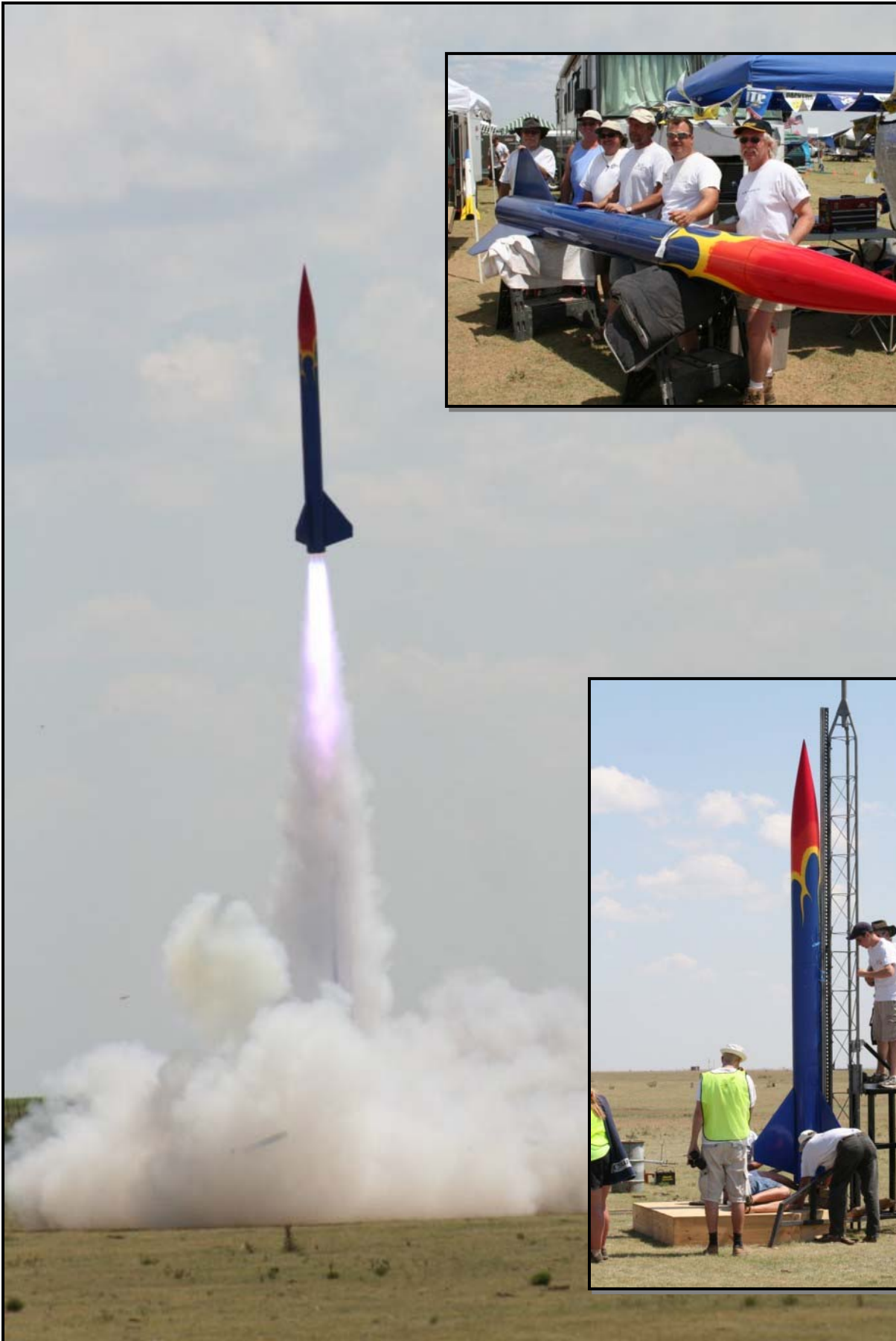
Tim Lehr and his Team Wildman flew their rocket The Wildman on a cluster of seven AMW Blue Baboon motors: an N2700, three M1900's, and three L1080's; this was one of the most powerful flights at LDRS 25.
