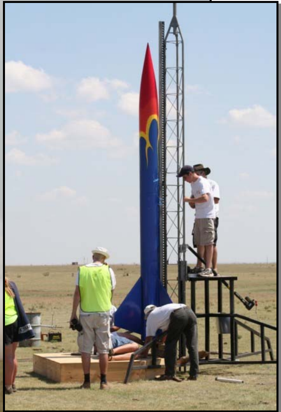
Tim Lehr and his Team Wildman flew their rocket The Wildman on a cluster of seven AMW Blue Baboon motors: an N2700, three M1900's, and three L1080's; this was one of the most powerful flights at LDRS 25.
