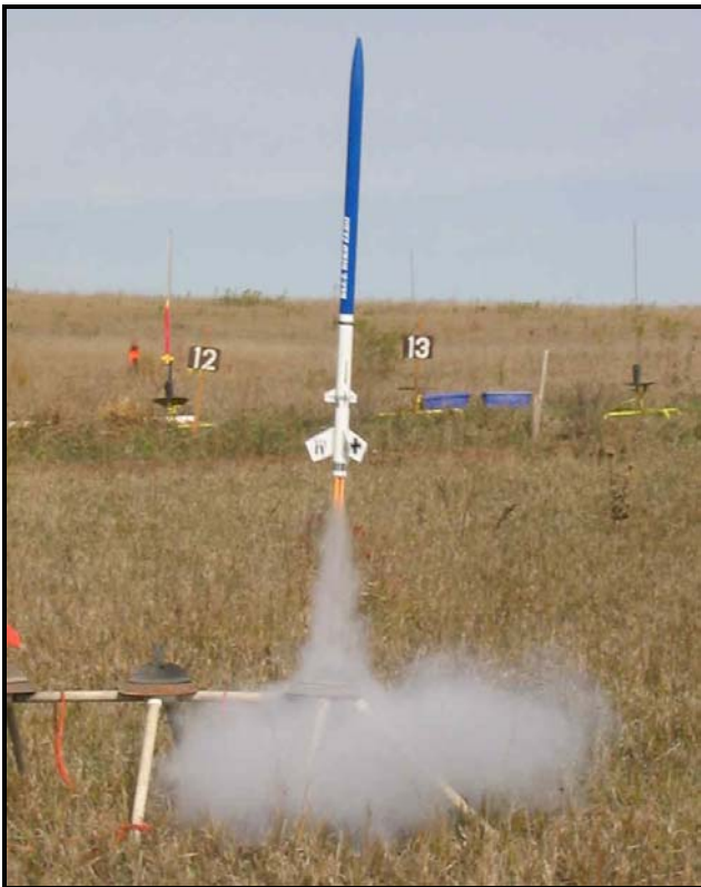
Liftoff on a cluster of three C6-3's. (Burney)
