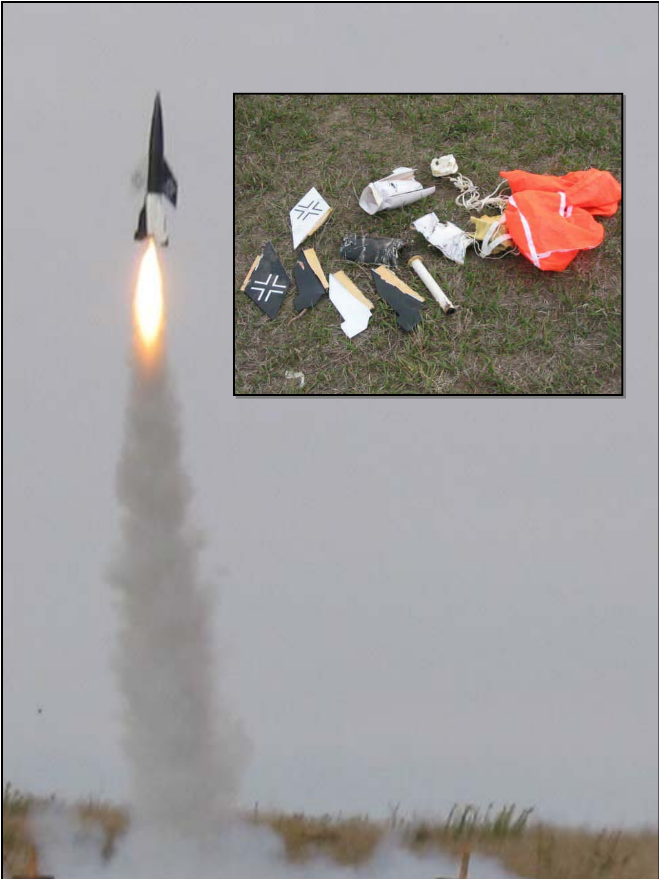
In Doug's case, his A4b's flight wasn't so smooth. The H180's ejection charge failed resulting in a core sample. With most of the fins salvageable, Doug hopes to rebuild. (Burney)
