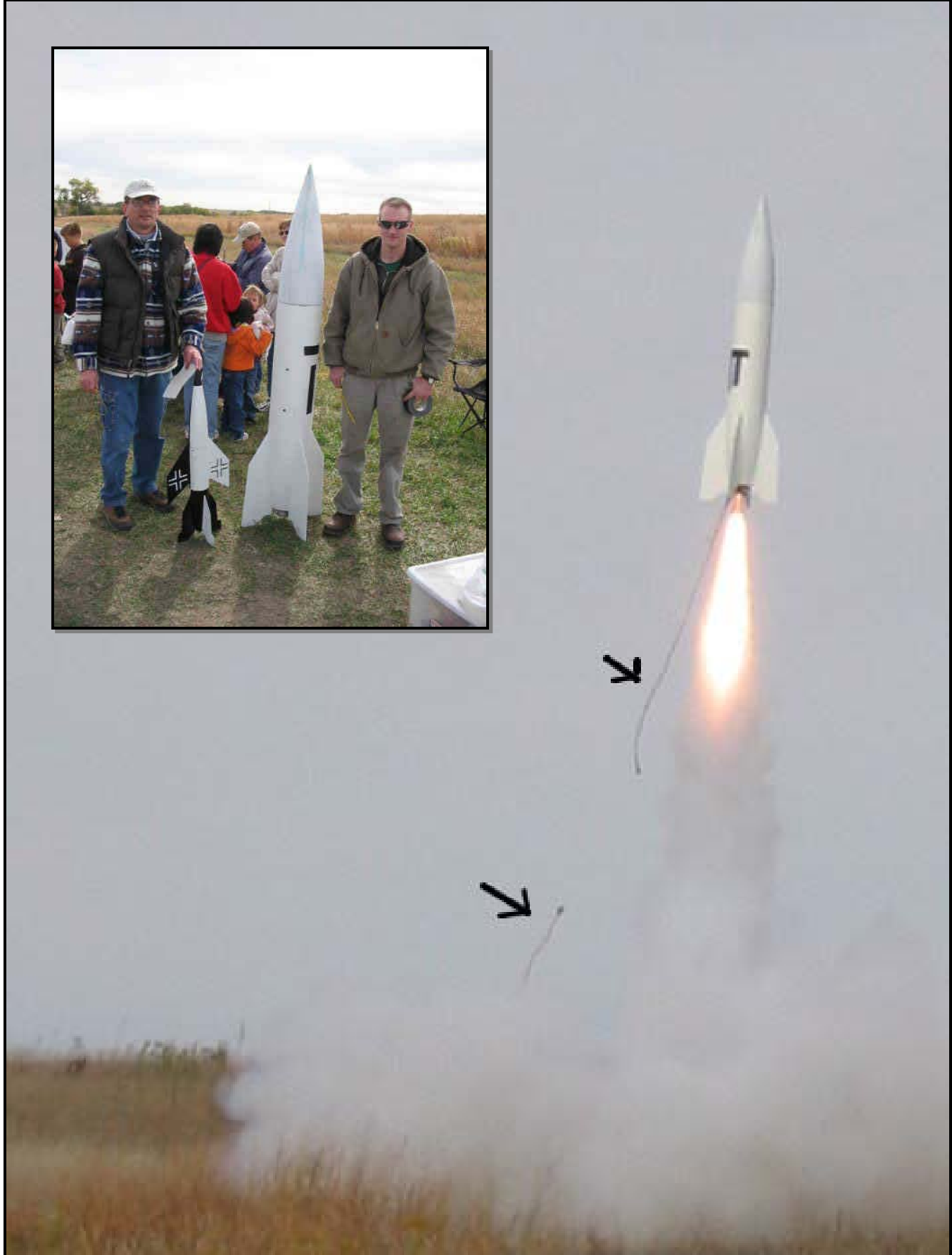
Inset: Doug Gard with his A4b (winged V-2) and Matt Jones with his own V-2. Matt flew his V-2 on an Animal Motor Works L777. The arrows point to the trailing igniter leads and extension cord. (Burney)
