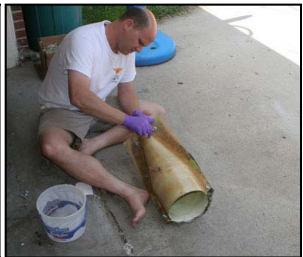
(Right) The 24" main nosecone after sanding. Matt really enjoyed working on this, as it provided the opportunity to pack about 2 pounds of foam shreds into the treads on his shoes, so that he could track it all over the house, before realizing it was there. Note the "precision crafted tool" Matt used for delicately shaping the main nosecone. (Right) Bolting the mold halves together, so that a layup can be done over the seam, then it goes back into the redneck oven until the nose is fully cured. Notice the strict adherence to OSHA guidelines, especially in terms of the non-slip footwear?
