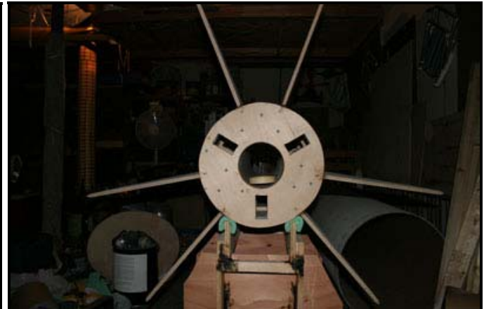
(Left) Semi-side view of the main motor mount. The 1x2 strips between the centering rings are to provide support while the entire assembly is slid into the airframe. This reduces the pressure on the motor tube which, being phenolic, is subject to cracking or breaking under too much stress. (Right) A whole lotta fins goin' on... It's starting to look like a rocket!
