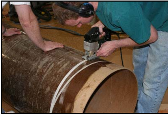
(Left) Matt cutting the end off of the 24in upper tube. (Right) Cutting fin slots. Do you know how much fun it is to draw straight lines on a 108" long tube?
