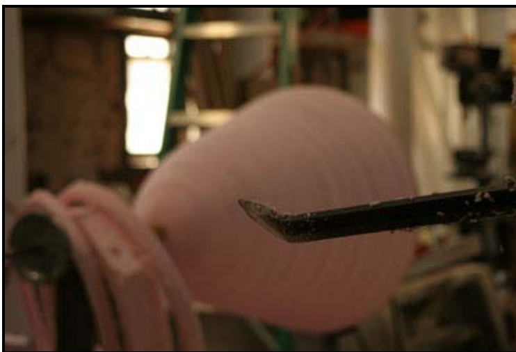
(Right) The 24" main nosecone after sanding. Matt really enjoyed working on this, as it provided the opportunity to pack about 2 pounds of foam shreds into the treads on his shoes, so that he could track it all over the house, before realizing it was there. Note the "precision crafted tool" Matt used for delicately shaping the main nosecone. (Right) Bolting the mold halves together, so that a layup can be done over the seam, then it goes back into the redneck oven until the nose is fully cured. Notice the strict adherence to OSHA guidelines, especially in terms of the non-slip footwear?
