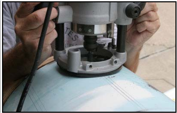
(Left) Matt cutting the end off of the 24in upper tube. (Right) Cutting fin slots. Do you know how much fun it is to draw straight lines on a 108" long tube?
