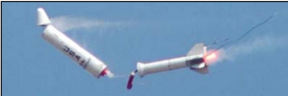
The altimeters fire the recovery charges. Yes, it's supposed to come apart like that. Though the main booster section was severely damaged due to the chutes stripping, Kevin and the rest of the team plan on rebuilding it and flying it at LDRS near Amarillo, TX next summer!
