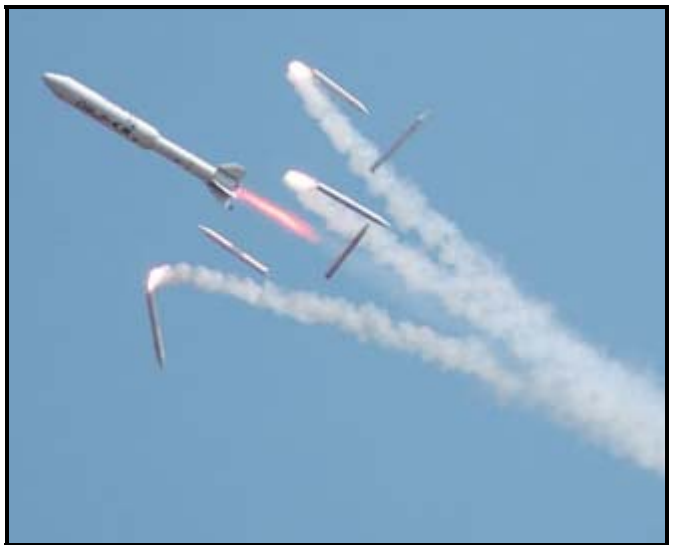
(Left) The first 3 boosters separate. (Right) The remaining 6 boosters separate.
