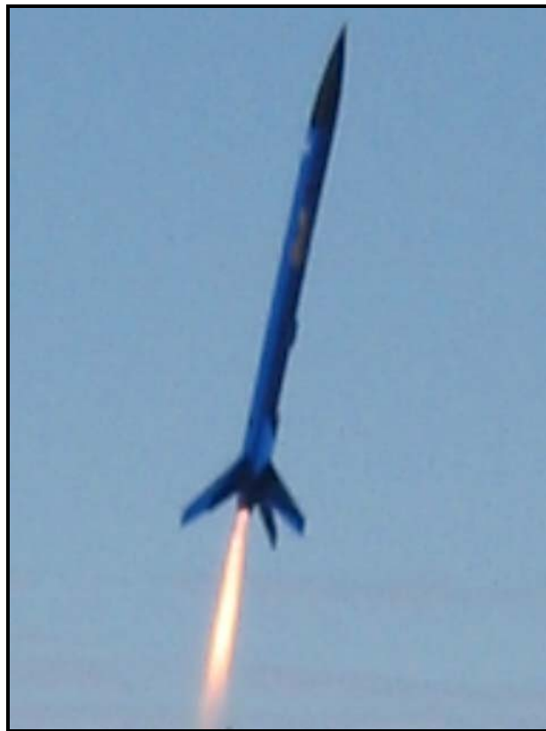
Liftoff on a Pro38 I205. As a result of the motor chuffing, the delay element was extinguished and the rocket core sampled. (Burney)
