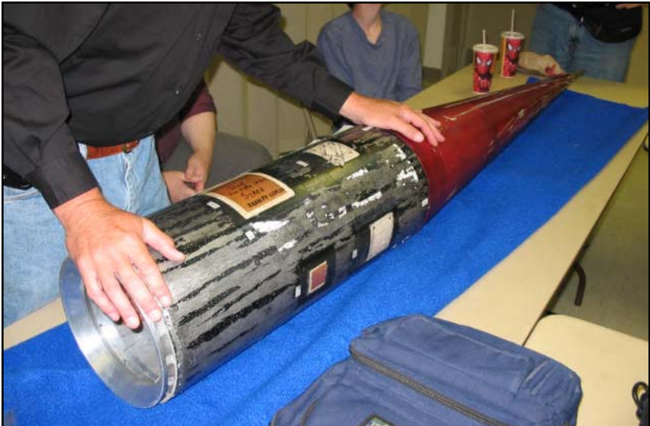
The payload section of the Civilian Space eXploration Team (CSXT) rocket. (Burney)
