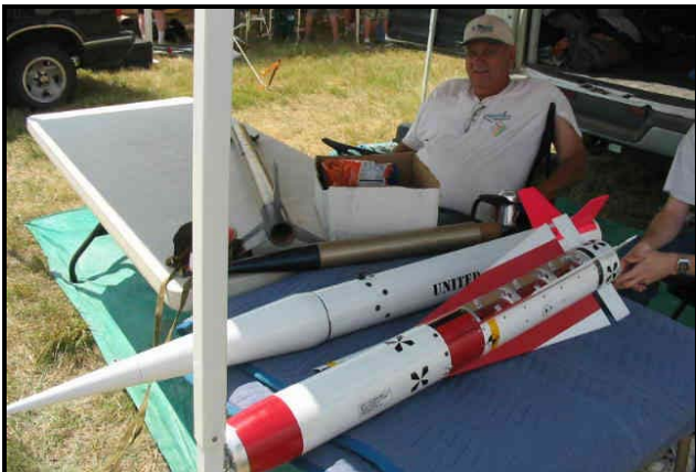
Larry Mills and his Nike Smoke and Maverick. Both rockets are all-aluminum construction! Note the removed panel on the Maverick revealing the AeroTech 1706 motor case!
