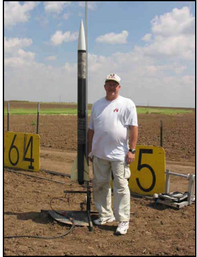
Bill Richardson and his carbon-fiber finished PML Endeavor. A Pro54 L730 took it to over 9,700'! Bill's highest flight yet!
