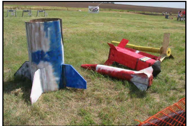
All of the finished rockets. The big blue rocket's nose is formed by folding up the top!
