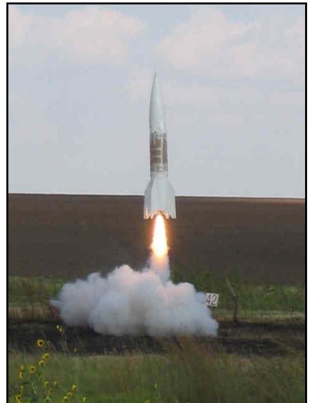
This 1/4 th scale V-2 was made mostly from cardboard and was flown several times on Saturday. This flight was on a J415.
