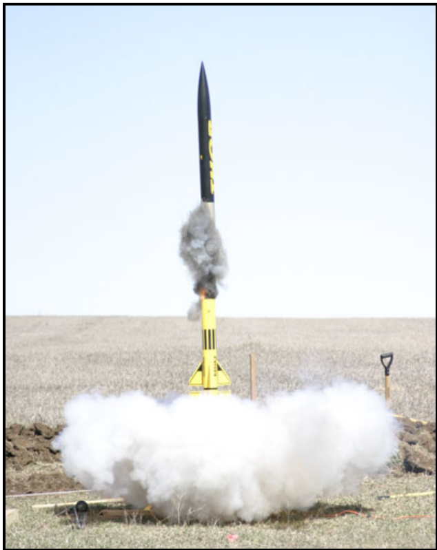
Within a fraction of a second of ignition, the J350 and its motor adaptor punched its way up through the rocket. (Jones)
