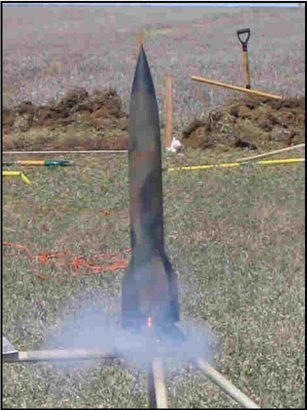
Mark's V-2 at the moment of ignition on a D12-3. The small motor combined with the winds resulted in a cruise missile flight trajectory. (Smith)
