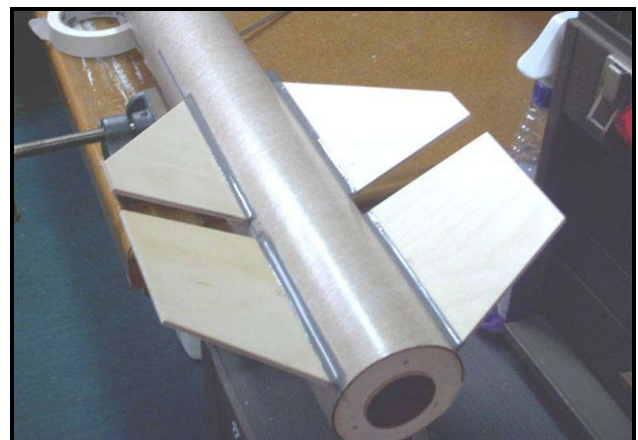
Nearly complete booster section. (Michel)
