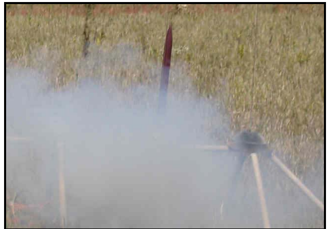
At ignition, Bridge's Skydiver was suctioned to the blast deflector. The Bernoulli Effect in action!
