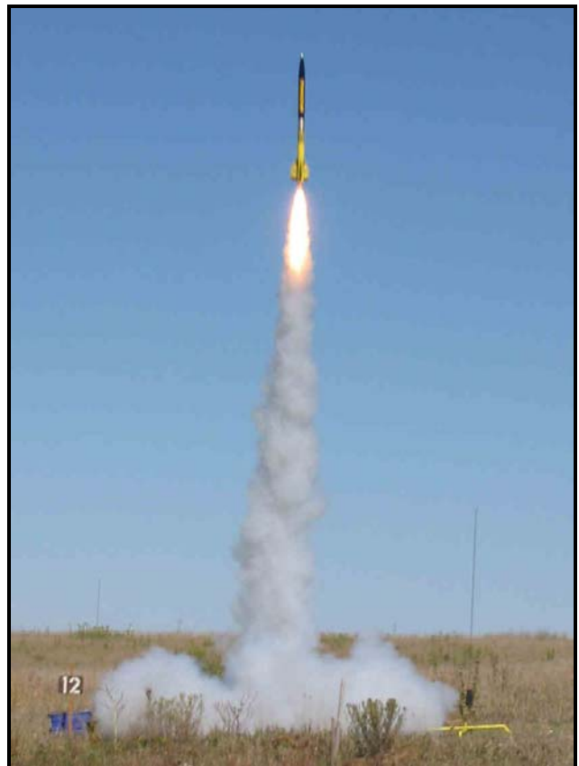
A J350 took Joe's THOR to 4,266 feet. This time the dual-stage deployment worked without a hitch. Awesome flight, Joe! (Burney)
