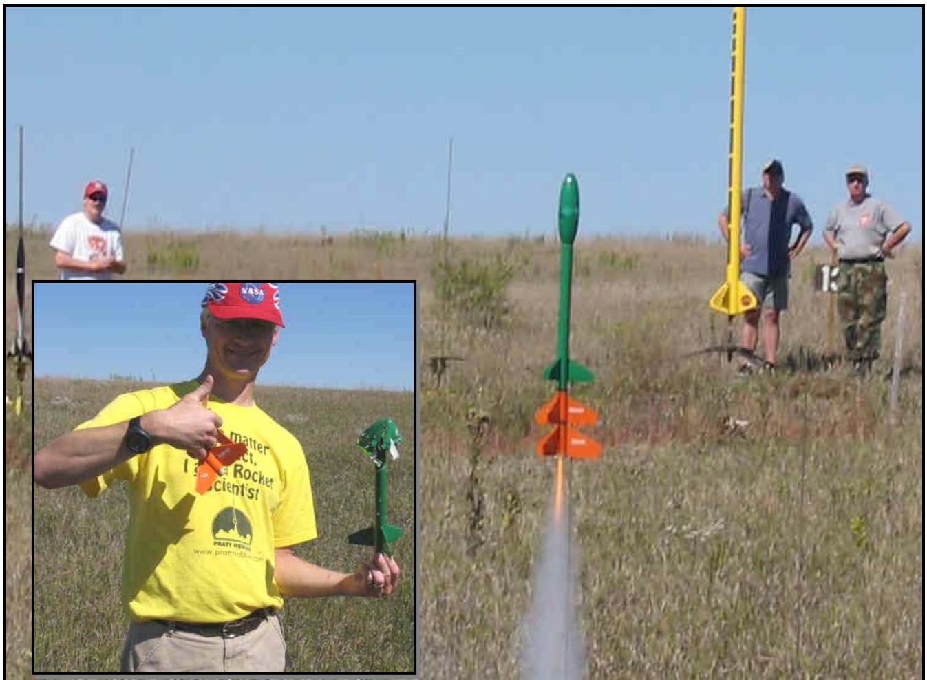
Skip Legge's PKT 1-2-3 lifts off on a C11-0 (C6-0 and C6-5 for stages two and three) with an egg for a payload. Inset – Skip just made scrambled eggs the hard way! The C6-0 second stage failed to light resulting in a lawn dart and a goey mess. (Richard Burney)
