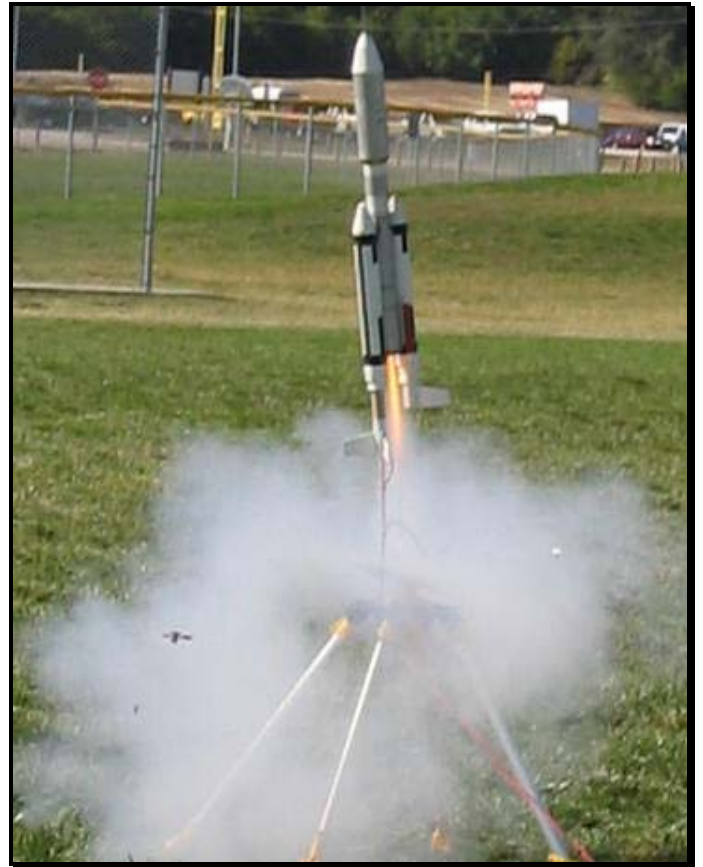
Spectacular shot of my Titan IIIE being stuck on the pad due to the wires catching a fin pod. Talking about a major waste of a perfectly good D12!
