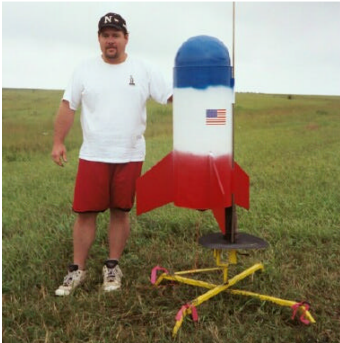
Mark Havel's rocket, though standing only about 42 inches tall, has the distinction of being one of the widest (13 inches) ever flown at a THOR launch. The nose cone was from a garbage can lid!
