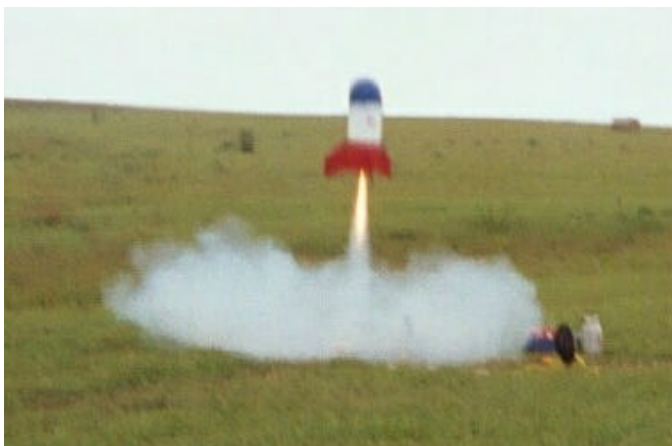
Mark flew his rocket on a Pro38 I285. Since the rocket weighed about 15 pounds, the I285 took the rocket up to only about 200 feet.
