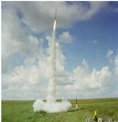
Final Fantasy VII heads up to over 4,200 feet via a J350. A broken shock cord resulted in a hard landing for the booster section.
